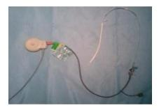
Make sure the Toco lead for external monitoring is used as pictured
